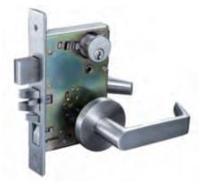
American Standard Function 7092: X=70mm Centre Distance:92mm,Backset:70mm Material : Stainless steel Finish : Satin Stainless steel Suitable for door thickness:44-57mm Suitable for : Interior door locks ,swinging door handle locks.
