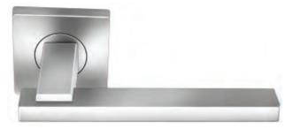
Specifications Material: Stainless Steel Door Thickness: 35-55mm 8mm Sprung covered Rose Bolt through fixings and SS 304 screws supplied
